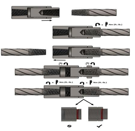
NOTE :Couplers must be assembled with calibrated torque wrench. Torque wrench must be
